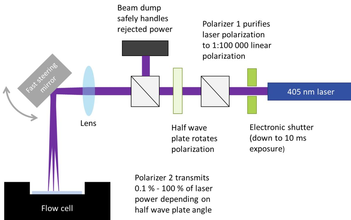
Figure 2 - Schematic of the laser scanner
