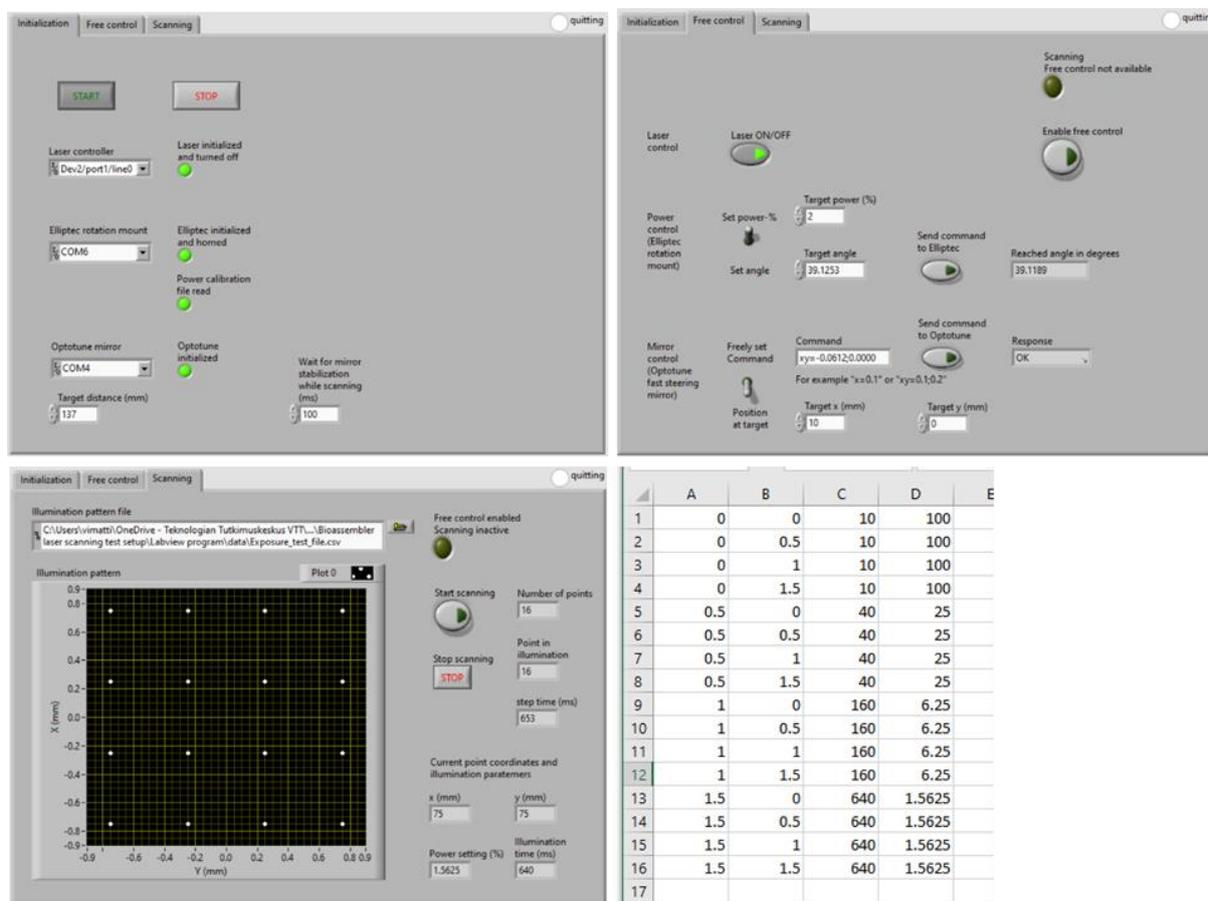
Figure 7 - LabVIEW user interface and test exposure file with position in x (mm), position in y (mm), exposure time (ms) and laser power (%) as the columns.
