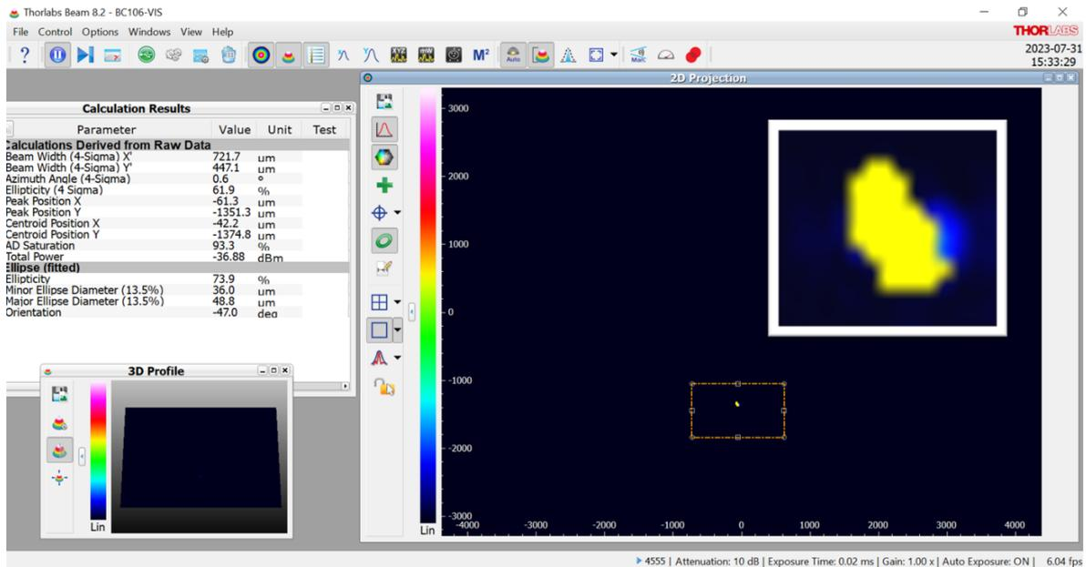
Figure 5 - Beam camera image of the laser spot in focus. Due to 5 µm pixel size of the camera, beam characteristics cannot be very accurately determined.
