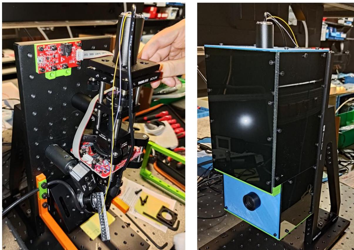
Figure 3 - Photographs of the laser scanner without and with laser safety enclosure.
