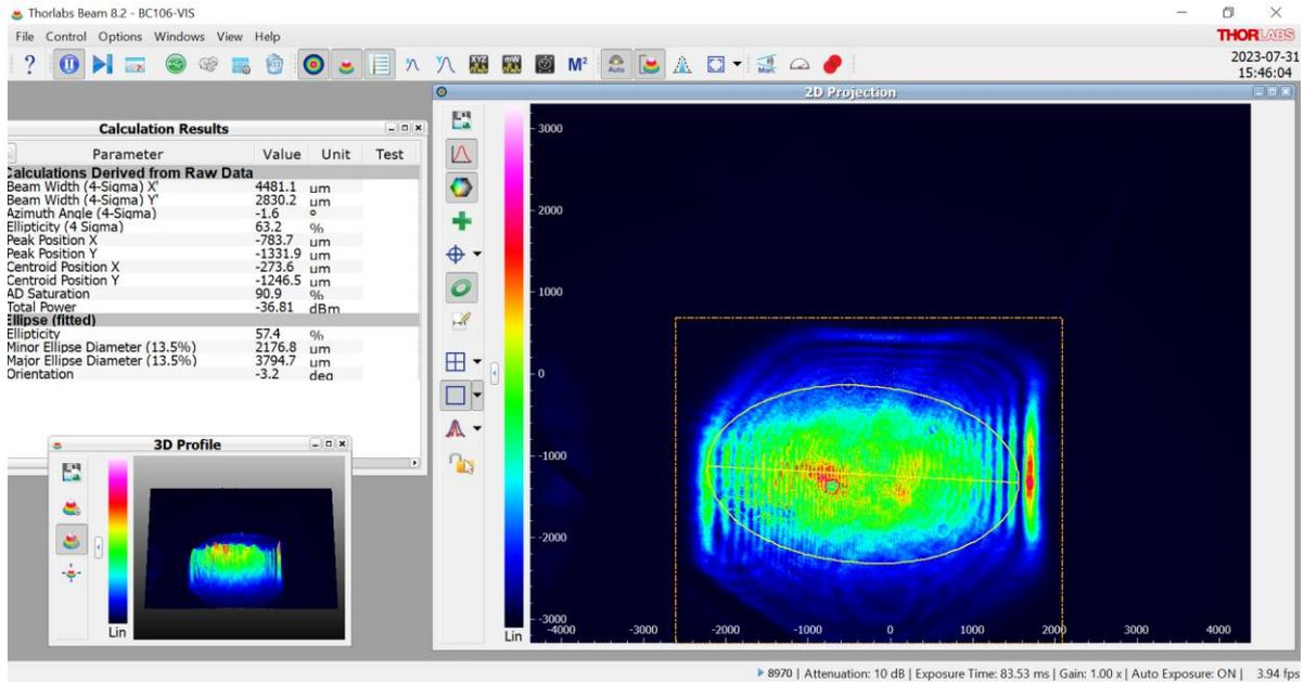
Figure 4 - Beam camera image showing the ellipticity of the laser beam and diffraction effects caused by 5 mm diameter polarizer.
