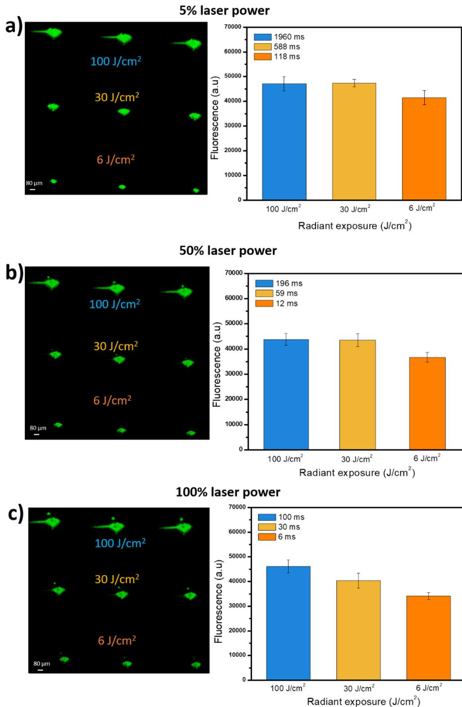
Figure 9 - Comparative study of exposure conditions used to synthesize a 25-mer sequence using the laser system. Different laser powers—(a) 5% (~51 W/cm<sup>2</sup>), (b) 50% (~511 W/cm<sup>2</sup>), and (c) 100% (~1022 W/cm<sup>2</sup>)—were used to synthesize the sequence using radiant exposures of 6, 30, and 100 J/cm<sup>2</sup> with different exposure times.
