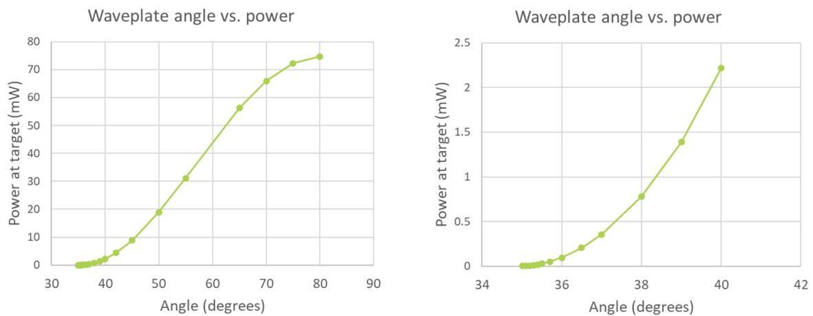
**Figure 6 - Data used for power calibration. Laser scanner software calculates the required waveplate angle using the calibrated data when desired power level in percentage of maximum power is given.**
