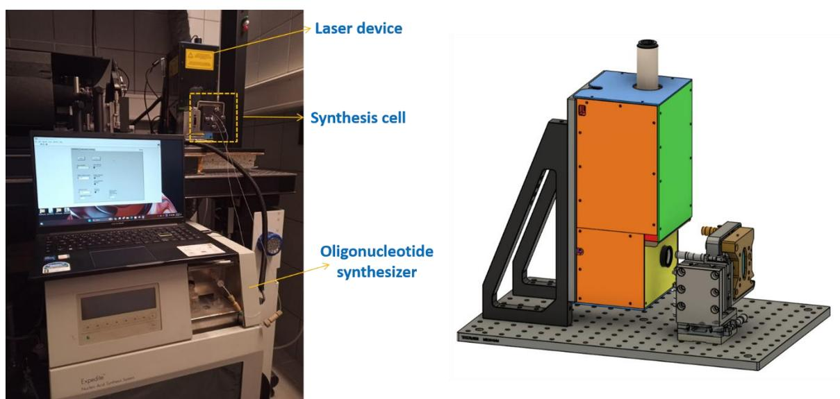
Figure 8 - Photograph of the fully assembled system for laser-based DNA synthesis along with a scheme of the optical system assembled on a breadboard. The fluidics delivery, an Expedite 8909 nucleic acid synthesizer, is connected to the fluidic cell positioned at the focal point of the laser. Also visible is the control computer which is connected to the laser system.
