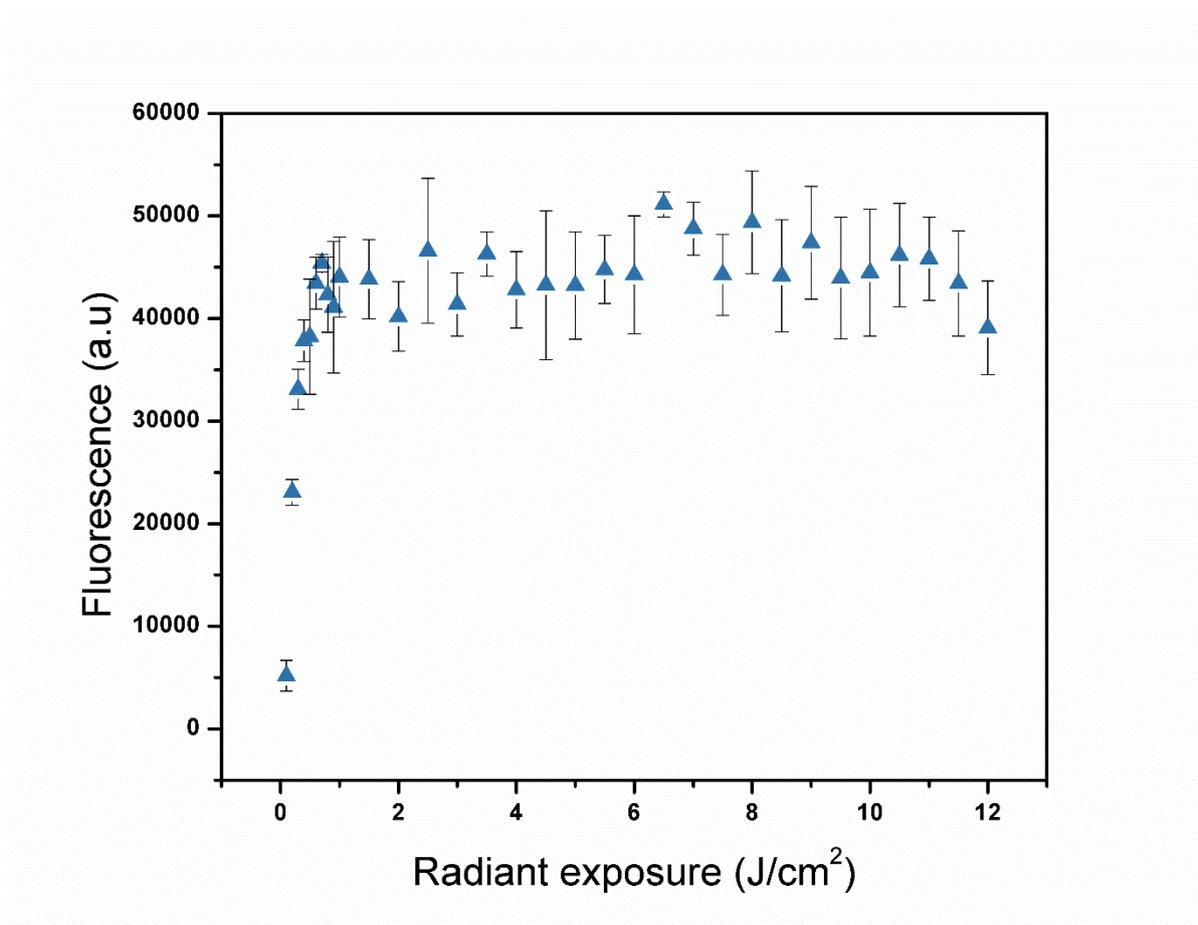
Figure 10 - Hybridization intensities for 25-mer sequence arrays were synthesized with an exposure gradient. The synthesis was done using 5% and 1% laser powers, with exposure times ranging from 10 to 235 ms. The signal intensities correspond to the average of five features.
